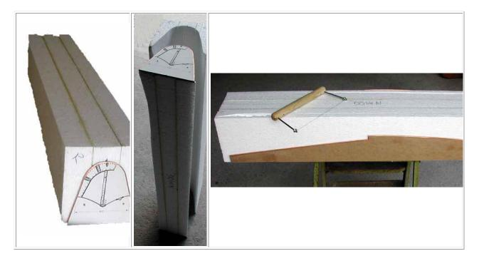
The fundamental difference cutting this style of foam core is the very first step. Templates of the same size and shape are nailed to the back and front of the foam core blank. The hot wire is run around the templates to cut out the equivalent of a "railroad tunnel". The "railroad tunnel" is tacked back onto the hump shape and the fat and thin side templates are tacked onto the outer sides of the "railroad tunnel".
