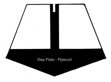
As Phil Peloquin points out, when all is said and done, it all happens on the step. This area takes the most punishment and some reinforcement might be appropriate. The simplest method is to insert a light plywood step plate.
