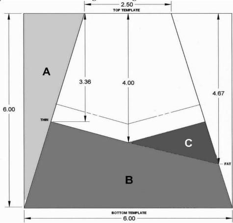
The first two first two cuts will have removed the material shown as "A" on the left side - and its mirror image on the right.
