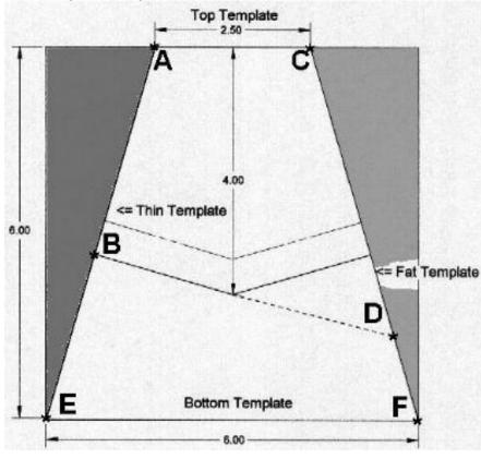
The top template will follow the exact shape of the foam core that we wish to emulate. Since the foam core is going to be covered with1/16 thickness balsa, we must make the foam core 1/16 smaller than the finished product on all sides. Having traced out the shape of the upper surface we must now employ some of our high school geometry to figure out with the bottom template should look like. In essence, we have to project the sides to a shape that is considerably larger than
