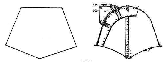
It is suggested that the EDO<sup>™</sup> pattern is a bit more difficult and should be attempted only after the basic CG /GP<sup>™</sup> patterns have been mastered. In our hobby, floats are sized to match two-cycle engine bores of 25, 40 and 60 cu. inches. The 40 size, or 36-in. length, is the most popular. The bulk of this article will assume that we are going to make the basic 36 in. CG /GP<sup>™</sup> pattern. Afterwards, we will have a quick look at the EDO<sup>™</sup> style.
