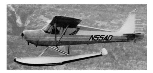
The aircraft in the photo above is a real Arctic Tern. Take careful note of the datum line running through the length of the fuselage and its relative angle to the line running along the top of the float. That works for this specific aircraft. Other aircraft do not require the same dramatic float tip droop.
