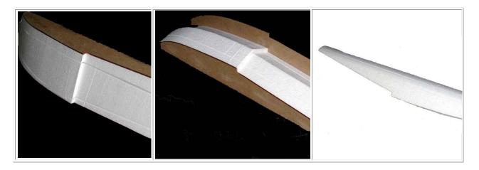
Once the first cut is made, the fat and thin side templates are reversed and a second cut made to get a perfect "Vee". The result is shown above.
