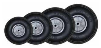
"SkyLite" Light Weight Wheels. Made with a unique molding process, "Skylite" wheels have a light urethane foam interior covered with a smooth, tough outer skin. As a result, these realistic looking wheels are unusually light yet highly resistant to wear and compression set. No inflation is required. Nylon hubs may be drilled out to the next larger axle size.
