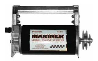
*Mariner.* Heavy duty starter made for starting boat engines with starter belts. Top handle with switch. Aluminum Double Pulley Drive Cone. 12 or 24 Volts with a maximum of 100 Amps. 600 in-oz of torque on 12 Volts, 1200 in-oz on 24 Volts. 2800 no load RPM. No. S650
